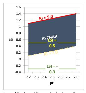
Figure 1. Comparison of Preferred Ranges in the Langelier and Ryznar Indexes
